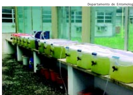
Testes em campo simulado avaliaram a atividade de larvicidas microbianos SIMULATED FIELD TESTS EVALUATED THE ACTIVITY OF MICROBIAL LARVICIDES
